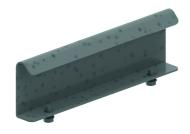
Joiner for HDKS HDSSU Tubular side walls. Perforated C-rungs 15x30 Usable inner height: 45 mm Rung distance: 250 mm
