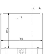
Build-in frame with border + tileframe + stainless steel cable outlet
