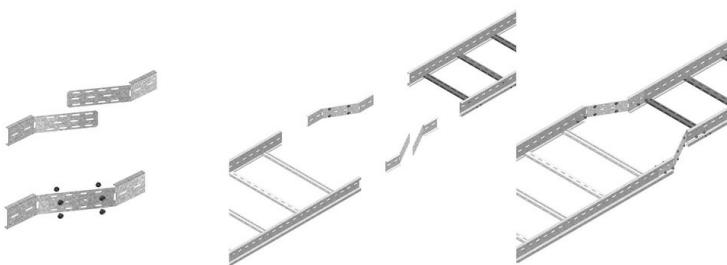
**A fixer avec:**
